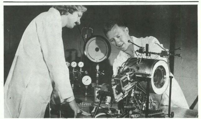
PREPARING THE "COMBUSTION BOMB" for a series of tests using fuel-injection are Mike Dyer (8116), left, and Udo Renger, an engineer from Volkswagen Research in West Germany. The stratified charge engine simulator incorporates two windows for making high-speed optical measurements of the combustion process.
